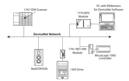
• Cost-effective wiring – one wire supplies communications and 24V DC power.
