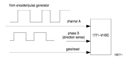
In this mode, direction (up counting or down counting) is determined by the channel B input, which can be an asynchronous signal.
