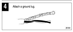
When using shielded cable wire, ground the foil shield and drain wire only at one end of the cable. We recommend that you wrap the foil shield and drain wire together and connect them to a chassis mounting bolt. At the opposite end of the cable, tape exposed shield and drain wire with electrical tape to insulate it from electrical contact.
