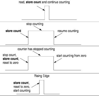
O You can also select these features using the falling edge of the gate/reset pulse. This selection is made through the gate invert bit, which is active in the store count and period/rate modes.
