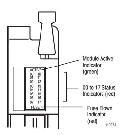
The front panel of your module contains one green, module active indicator, 16 red status indicators and one red fuse-blown indicator. The 1771-OMD/B performs diagnostics in a handshaking mode when first powered up. Upon successful completion of the diagnostics, the green module active indicator lights. It turns off if a fault occurs in the data paths or the opto-isolators.
