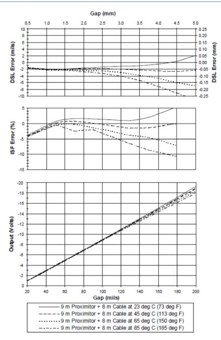
Figure 8: Typical 3300 XL 11 mm 9 m Proximitor with 8 m of Extension Cable @ High Temperature
