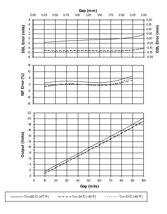
Figure 6: Typical 3300 XL 8mm 9 m Proximitor Sensor with 8m of Extension Cable at  $T_c$  (Probe is at 25 °C)
