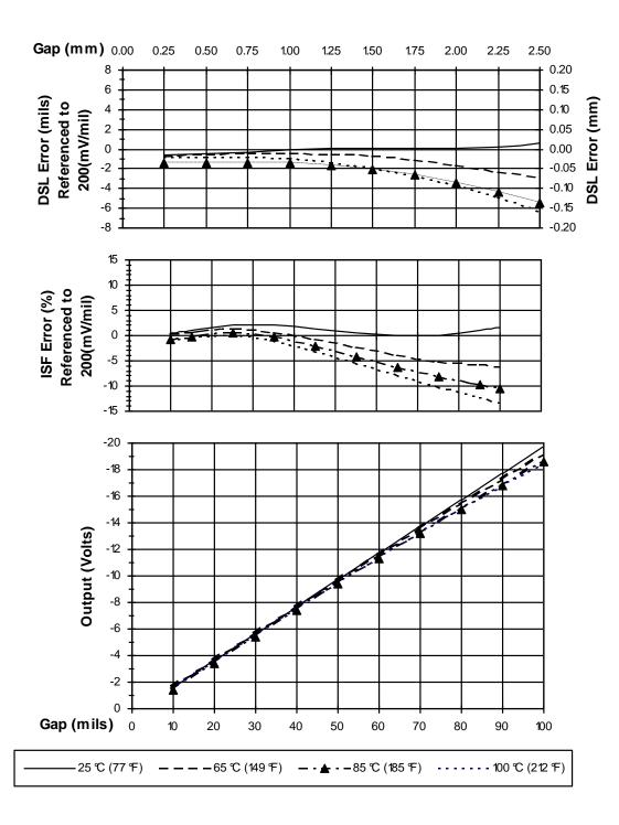
Figure 5: Typical 3300 XL 8 mm 5m Proximitor Sensor with 4m Extension Cable at Th (Probe is at 25°C)
