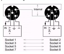
Two input signals can be connected to each input socket. If both inputs of the same socket are used. the other socket of the pair (1/2, 3/4, 5/6, 7/8) must not be used.
