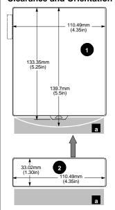
Carriers must be mounted on a horizontal DIN rail.
