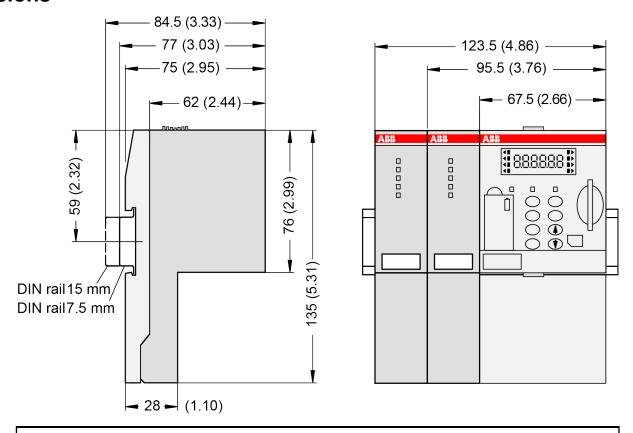
The dimensions are in mm and in brackets in inch.
