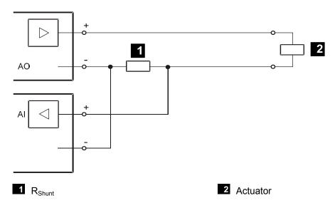
Figure 2: Application Example for Safety-Related Analog Outputs
