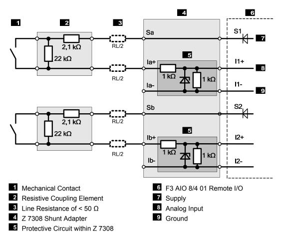
Figure 12: Mechanical Contact with Resistive Coupling Element
