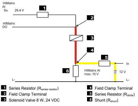
Figure 1: Circuitry for Line Monitoring
