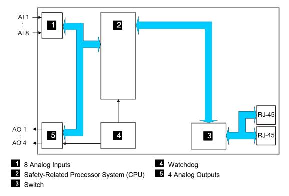
Figure 5: Block Diagram
