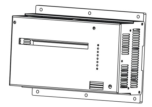
Figure 7: HIMatrix F3 AIO 8/4 012 with Aluminum Plate
