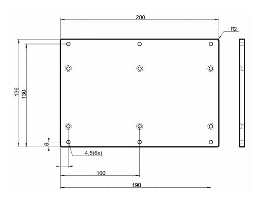
Figure 8: Aluminum Plate with Dimensions
