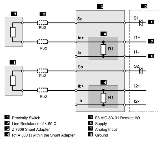
Figure 10: Proximity Switch on Analog Inputs
