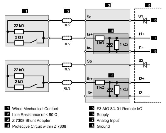
Figure 11: Wired Mechanical Contact
