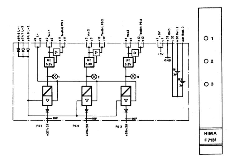
The module F 7131 monitors the system voltage 5 V generated by the 3 power supplies max. as follows:
