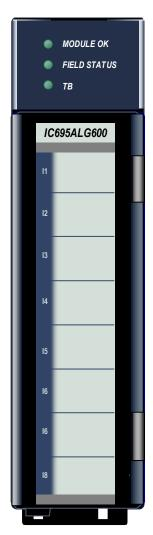
Universal Analog Input module IC695ALG600 provides eight general purpose input channels and two Cold Junction Compensation (CJC) channels. Inputs are divided into two equal groups of four. Channels can be individually-configured using the Machine Edition software for:
