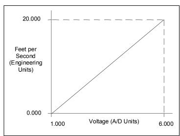
For this example, 1.0V to 6.0V is the normal voltage range, but the module will attempt to scale the inputs for a voltage that lies outside the range. If a voltage of 10.0V were input to the channel, the module would return a scaled channel value of 36.000. The application should use alarms or take other precautions for scaled inputs that are outside the acceptable range or invalid.
