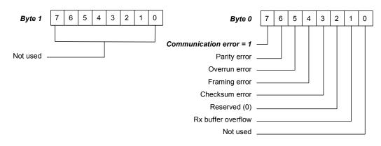
Error conditions include parity and overrun errors. In addition, a field device will report an overflow of its receive buffer, and any discrepancy between the message content and the received checksum.
