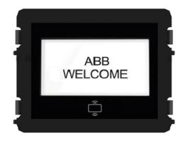
Display module for outdoor station which also doubles as a RFID card reader. It can be an ID card reader (125 kHz) or IC card reader (13.56 MHz) and is configured though the keypad module.
