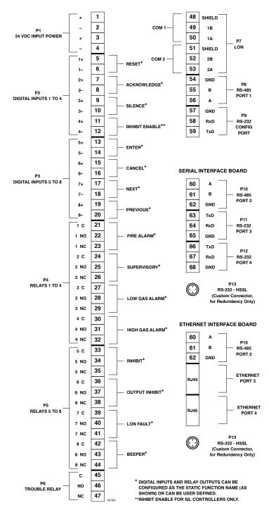
Figure 3-7—EQP Controller Terminal Identification
