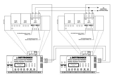
Figure 3-11B—Controller to Controller Communication with Class A Signaling Line Circuit Classification per NFPA 72, for Controllers with Ethernet Interface Board
