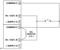
Figure 3-26—Supervised Input Configuration - Class A
