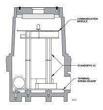
Figure 3-50—Printed Circuit Boards in Universal DCU
