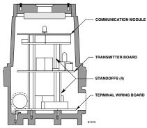
Figure 3-55—Printed Circuit Boards in Combustible Gas DCU
