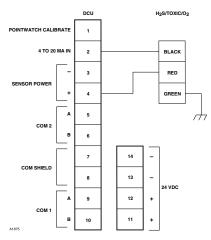
Figure 3-52—Electrochemical Sensor Connected to DCU
