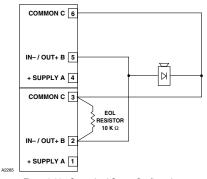
Figure 3-33—Supervised Output Configuration (Notification)— Class A
