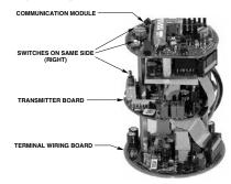
CORRECT ORIENTATION OF TRANSMITTER BOARD
