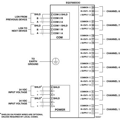
Figure 3-37—DCIO Module Wiring Terminal Configuration
