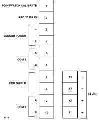
Figure 3-51—Wiring Configuration for DCU
