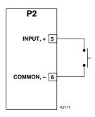
Figure 3-4—Unsupervised Input Wiring
