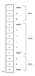
Figure 3-3—Network Extender Wiring Terminal Identification
