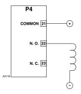
Figure 3-5—Unsupervised Relay Output
