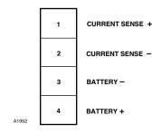
Figure 3-20—J2: Battery Test Points
