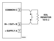
Figure 3-39—Supervised Input Configuration
