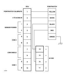
Figure 3-53—PointWatch/DuctWatch Connected to DCU
