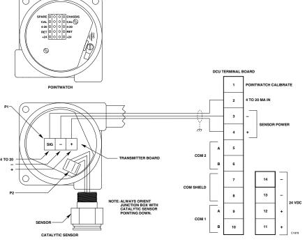
Figure 3-56—Sensor Separation Kits
