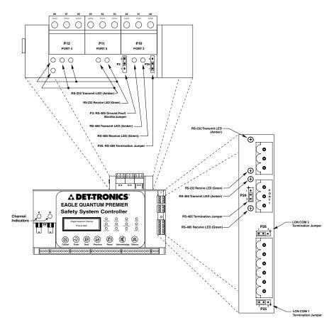
Figure 3-10A—Location of Termination Jumpers, Communication Indicator LEDs, and Communication Ports for Controller with Serial Interface Board
