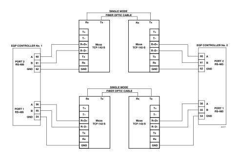
Figure 3-13—Single Mode Controller to Controller NFPA 72 Approved Fiber Optic Link, Class X
