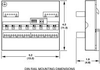
Figure 6-3—Dimensions of the EDIO / DCIO / Relay Module / AIM in Inches (Centimeters)
