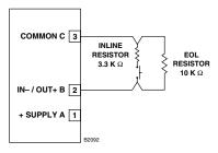
Figure 3-40—Supervised Input Configuration (Opens and Shorts)
