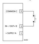
Figure 3-38—Unsupervised Input Configuration
