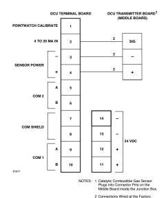
Figure 3-54—DCU Transmitter Board Connected to Terminal Wiring Board
