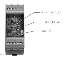
Figure 4-11—Ground Fault Monitor Status Indicator Location
