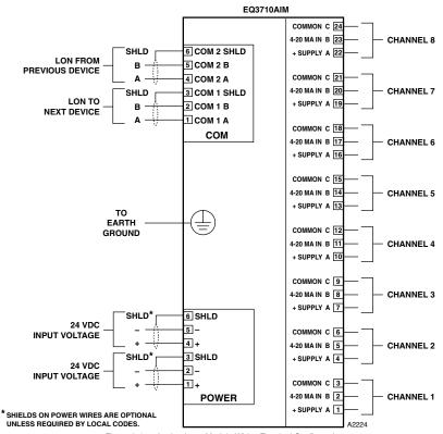
Figure 3-45—Analog Input Module Wiring Terminal Configuration
