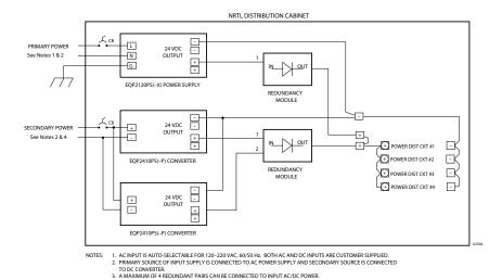
Figure 3-21C—Wiring Connections for a 20amp (Maximum) Power Supply with an AC Primary and DC Secondary Source
