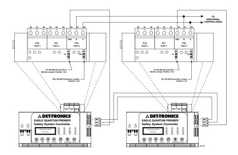
Figure 3-11A—Controller to Controller Communication with Class A Signaling Line Circuit Classification per NFPA 72, for Controllers with Serial Interface Board
