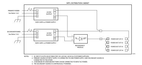
Figure 3-21A—Wiring Connections for a 20amp DC (Maximum) Power Supply with Primary and Secondary AC Sources
