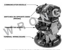
INCORRECT ORIENTATION OF TRANSMITTER BOARD
