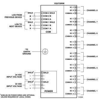
NOTE: RELAY CONTACTS SHOWN IN REST (DE-ENERGIZED) STATE.
