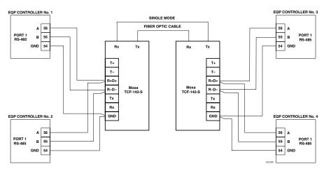
Figure 3-12—Controller to Controller NFPA 72 Approved Fiber Optic Link, Class B
