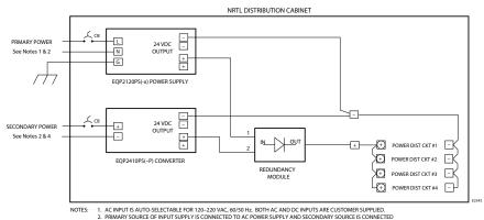
PRIMARY SOURCE OF INPUT SUPPLY IS CONNECTED TO AC POWER SUPPLY AND SECONDARY SOURCE I TO DC CONVERTER.
