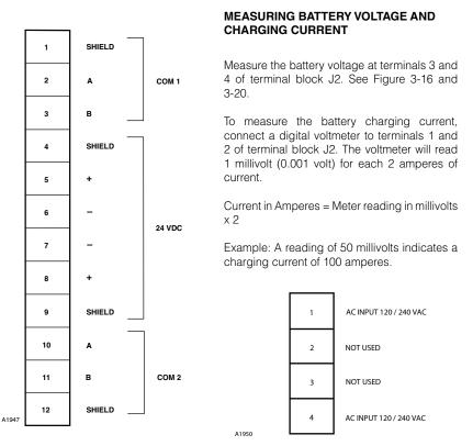
Figure 3-17—J1: Power and LON Wiring Terminal
