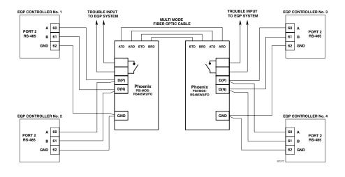
Figure 3-14—Multi-Mode Controller to Controller NFPA 72 Approved Fiber Optic Link, Class X
