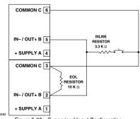
Figure 3-28—Supervised Input Configuration for Opens and Shorts – Class A
