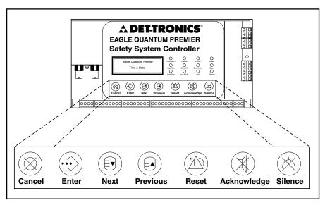
Figure 4-1—EQP Controller Pushbutton Locations
