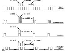
Figure 4-4—Tone Pattern for Controller Buzzer
