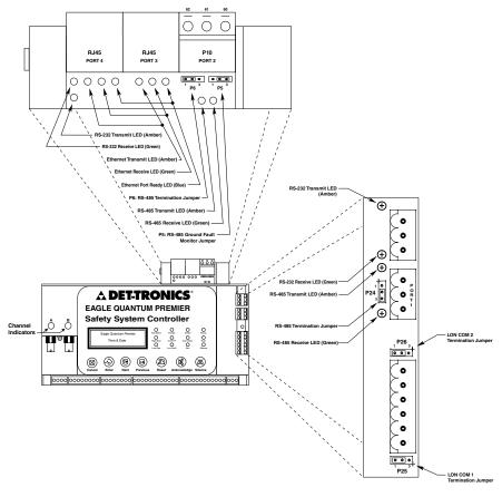
Figure 3-10B—Location of Termination Jumpers, Communication Indicator LEDs, and Communication Ports for Controller with Ethernet Interface Board
