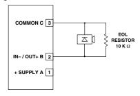
Figure 3-41—Supervised Output Configuration (Notification)
