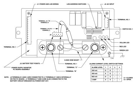
Figure 3-16—Power Supply Monitor Terminal and Switch Location
