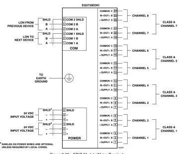
Figure 3-23—EDIO Module Wiring Terminals
