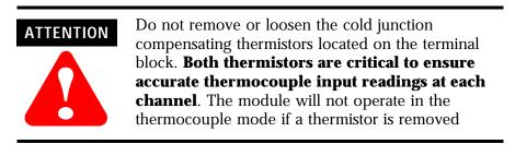
In case of accidental removal of one or both thermistors, replace them by connecting them across the CJC terminals located at the top and/or bottom left side of the terminal block. Always connect the red lug to the (+) terminal (to CJC A+ or CJC B+).
