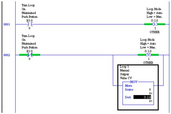
Figure 9.4 Correct way to shut down loop
