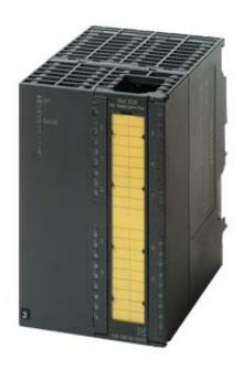
SIMATIC S7, DIGITAL OUTPUT SM 326, F-DO 8 X DC 24V/2A PM FAILSAFE DIGITAL OUTPUTS P-M SWITCHING UP TO CATEGORY 4 (EN954-1)/ SIL3 (IEC61508)/PLE (ISO13849), 1 X 40 PIN
